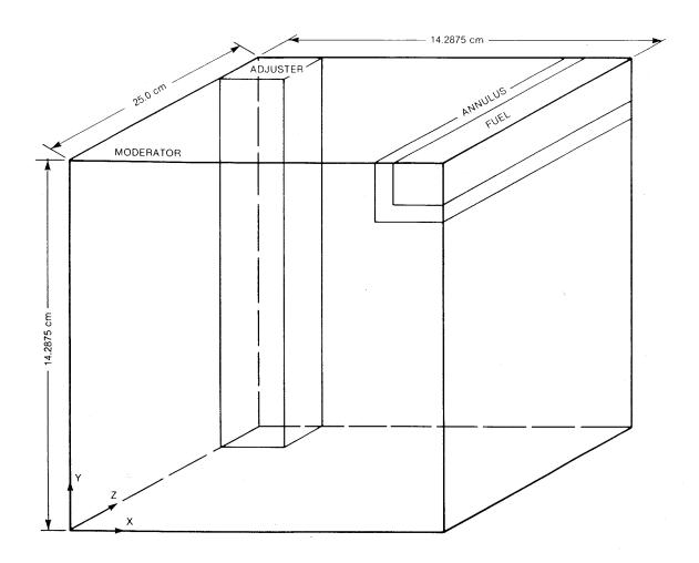
Figure 4.2a Typical RFSP Reactor Model (Face View)
